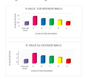
Figure 3: R-value for exterior and interior walls for rise buildings
