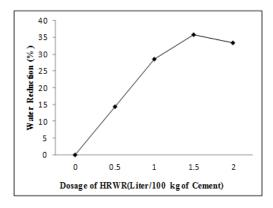
Figure 2: Relationship Between the Different Dosages of HRWRA and Water Reduction of Concrete Mix
