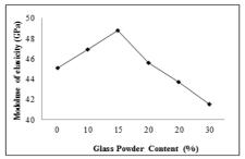
**Figure 6:** Effect of Glass Powder Content on the Static Modulus of Elasticity of Concrete.
