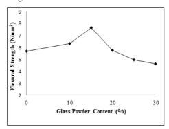
**Figure 5:** Effect of Glass Powder Content on Flexural Strength of Concrete.
