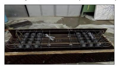
**Figure 2:** Peparation the mold specimen and placing the reiforcement
