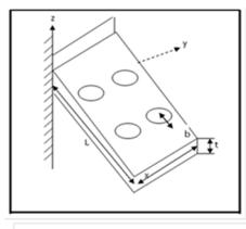
Fig. (1): fin with circular perforations
