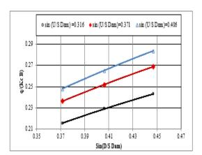
**Figure (6):** Relationship between (sin(D/S Dam)) and (q/kc B) of homogenous earth dam with core at U/S Core 1:2.5, D/S Core1:2.25
