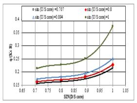
**Figure (4):** Relationship between (sin(D/S Core) and (q/kcB) of homogenous earth dam with core at U/S Dam 1:3, D/S Dam1:2.5
