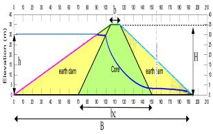
**Figure (3):** The general section of homogenous earth dam with core
