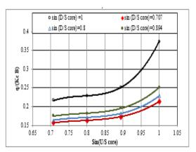
**Figure (5):** Relationship between (sin(U/S Core)) and (q/kc B) of homogenous earth dam with core at U/S Dam 1:3, D/S Dam1:2.5
