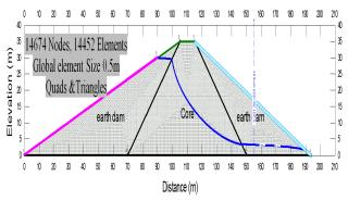
**Figure 2:** General Mash properties of homogenous earth dam with core
