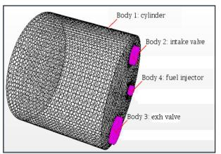
**Figure 3:** the mesh of the cylinder and valves
