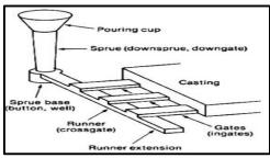
**Figure 1:** shows the ingates location in sand casting [2]
