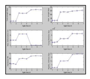
**Figure 8:** shows the effect of ingate area on mechanical properties
