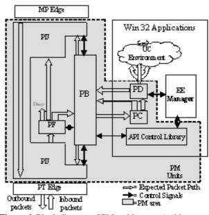
Figure 4. Block diagram of PM architecture Architecture
