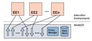
Figure 1. Active node architecture of DARPA
