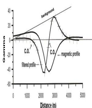
Fig.(2a) Magnetic anomaly profile for dyke-like body (depth 500, width 500, inclination angle 10°) with its filtered profile using Fraser filter.
