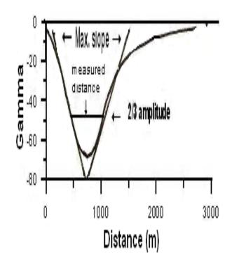
Fig.(5b) Residual curve obtained by subtracting Fraser filter values from background for the above magnetic profile.
