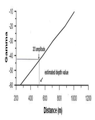
Fig.(4c) Depth estimation of dyke-like body from the relation of various amplitudes against distances between two straight lines of filtered profile.
