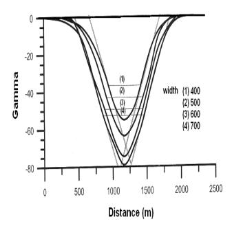
Fig.(6) Residual curve obtained by subtraction Fraser filter values from background for magnetic profile for dyke-like body with same depth of 500m, various widths and with inclination angle 400.
