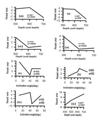
Fig.(7) Percent errors in depth estimation for dyke-like bodies a) same inclination with angle various depths, b) same depths and width with different inclination angles, c) same depth and inclination angle with different widths.
