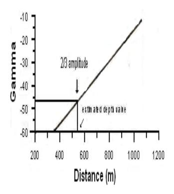
Fig.(5c) Depth estimation of dyke-like body from the relation of various amplitudes against distances between two straight lines of filtered profile.
