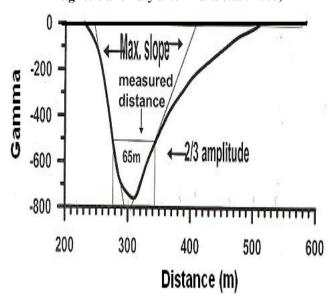
Fig.(8b) Residual curve obtained by subtracting Fraser filter values from background for magnetic field profile.
