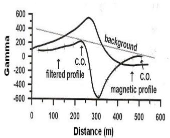
Fig.(8a) Field example of the total magnetic profile and its filtered profile obtained by applying Fraser filter. ( magnetic anomaly after Kara et.al. 2003)
