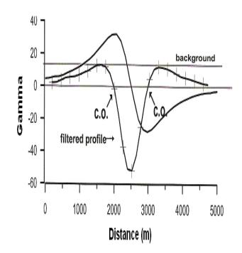
Fig.(4a) Magnetic anomaly profile for dyke-like body (depth 500, width 500, inclination angle 450) with its filtered profile using Fraser filter.
