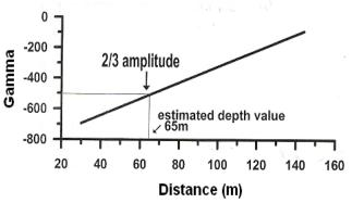
Fig.(8c) Depth estimation of magnetic source body from the relation of various amplitudes against distances between two straight lines of filtered field profile.
