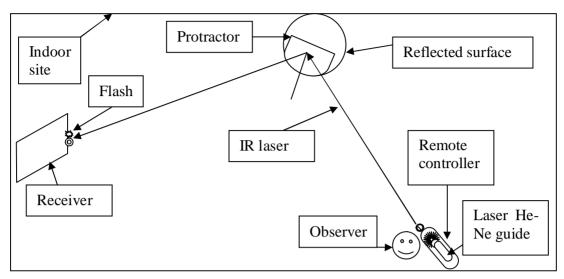
Fig.(1) schematic draw of reflected surfaces of IR laser signals from remote sensor to receiver in test site.
