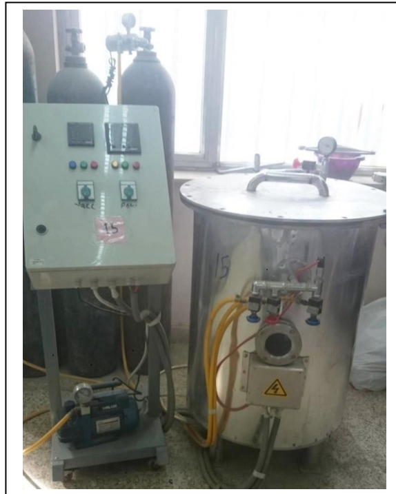
Plate 2. The CO 2 curing chamber
