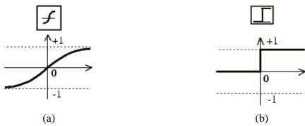
Figure (8): (a) hyperbolic tangent function. (b) hard limit function
