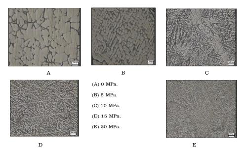
Figure (4) : microstructure of Al-5%Y\_2O\_3 prepared by squeeze casting.
