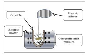
Figure (1) : stir mixer components.
