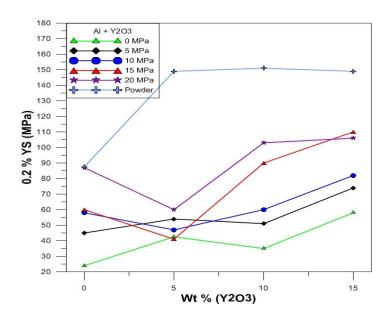
Figure (7) : effect of  $Y_2 O_3$  on compressive yield strength of Al-Y2O3 composites.
