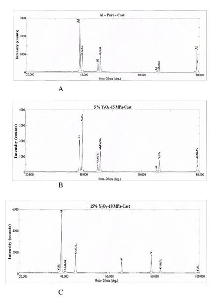
Figure (5) : XRD pattern of squeeze casting specimens (A) pure Al 0MPa (B) Al-5%Y\_2O\_3-15MPa (C) Al-15%Y\_2O\_3-10MPa
