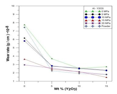
Figure (8) : effect of  $Y_2O_3$  on wear rate of  $Al\mathchar`-Y_2O_3$  composites.
