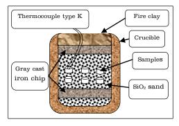
Figure (2) : sintering configuration.
