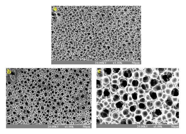
Fig. 2: SEM of PSi (a. without irradiated, b and c irradiated at 50 and 100 Gy respectively).
