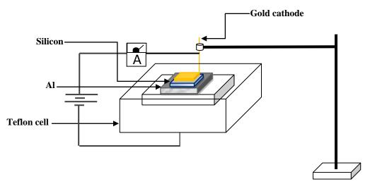
Fig. 1: Schematic electrochemical cell
