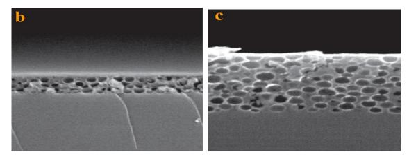
Fig. 3: Cross-sectional SEM images of PSi (a. without irradiated, b and c irradiated at 50 and 100 Gy respectively).
