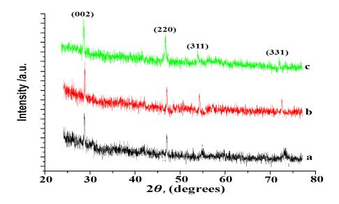
Fig. 4: XRD pattern of porous silicon (a) without irradiation, (b) after irradiation with γ- ray 50 Gy and (c) 100 Gy.
