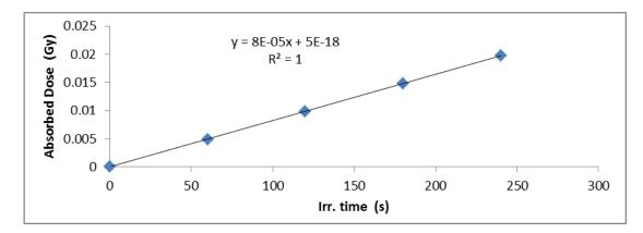
Fig.7: Relation between the absorbed dose in the irradiated nuclear track detector CR-39, and the irradiation time at constant etch time 8h, at angle 60°
