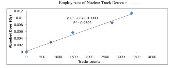
Fig. 9: Relation between the absorbed dose and tracks count at constant etch time 8h, at angle 30°
