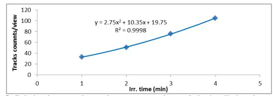
Fig. 5: Relation between the tracks counts per view and the irradiation time at constant etching time 8h, at angle 90°.
