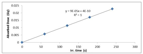
Fig. 8: Relation between the absorbed dose in the irradiated nuclear track detector CR-39, and the irradiation time at constant etch time 8h, at angle 90°
