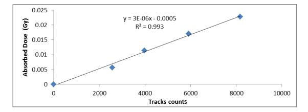
Fig. 11: Relation between the absorbed dose and tracks count at constant etch time 8h, at perpendicular angle 90°
