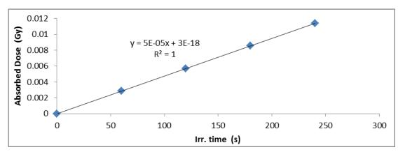
Fig. 6: Relation between the absorbed dose in the irradiated nuclear track detector CR-39, and the irradiation time at constant etch time 8h, at angle 30°
