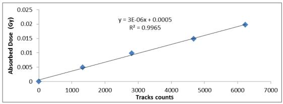
Fig. 10: Relation between the absorbed dose and track counts at constant etch time 8h, at angle  $60^{\circ}$
