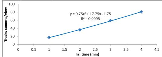
Fig. 4: Relation between the tracks counts per view and the irradiation time at constant etching time 8h, at angle 60°.
