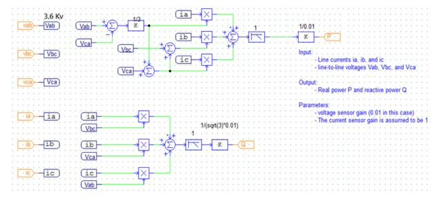
Figure 6: Switching-IGBTs controls P and Q
