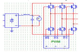
Figure 3: Converter-Circuit of Rectifier and Buck/Boost.
