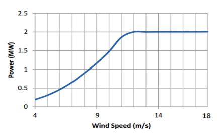
Figure 11: Power Curve for Simulated Model
