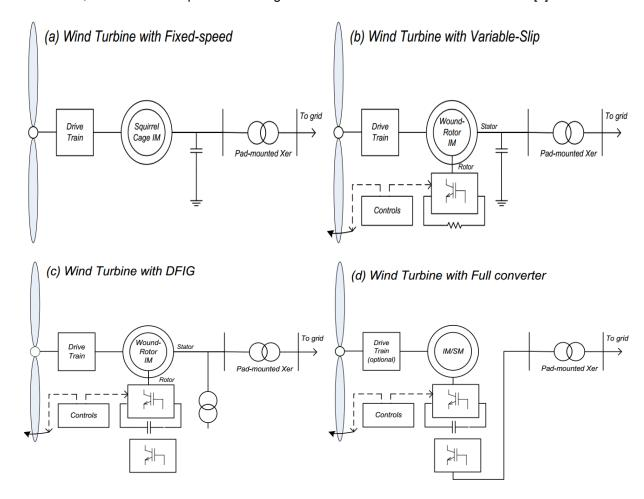
Figure 1. Wind Turbine Technologies [6]
