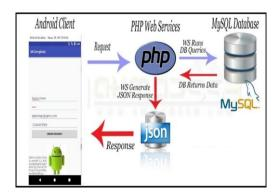
Figure 1. The architecture of the system
