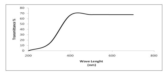
Figure(3-19)Transmittance of Copolymer(HEMA-co-MAA) in the visible light wave range of 400-700 nm
