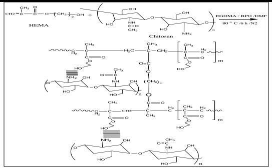
Scheme (3-2) Copolymerization and crosslinking of HEMA with Chitosan
