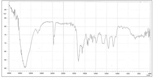
Figure (3-3):FTIR Spectra of Hydrogel (HEMA-co-Cs)
