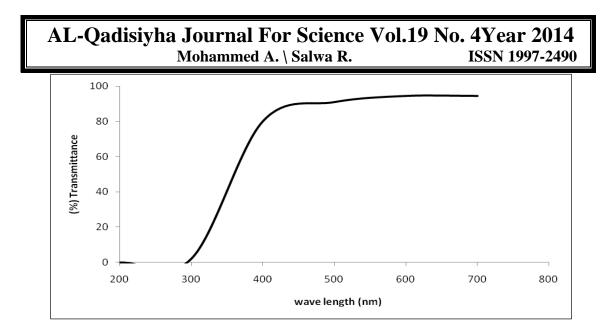
Figure (3-18) Transmittance of Copolymer (HEMA-co-MA) in the visible light wave range of 400-700 nm
