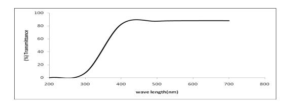
Figure(3-20) Transmittance of Copolymer (HEMA-co-EHMA) in the visible light wave range of 400-700 nm
