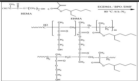
Scheme (3-3) Copolymerization and crosslinking of HEMA With Ethylhexyl methacrylate
