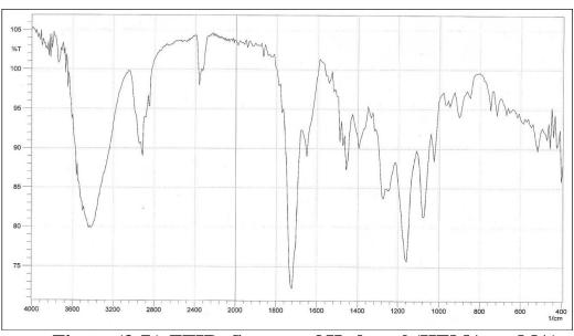
Figure (3-7):FTIR- Spectra of Hydrogel (HEMA-co-MA)
