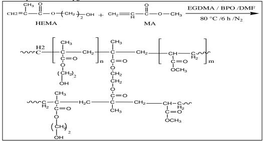
Scheme (3-4) Copolymerization and crosslinking of HEMA with methacrylate
