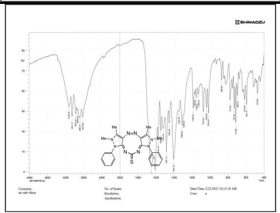
Fig. (4) : FTIR spectra of A4 compound
