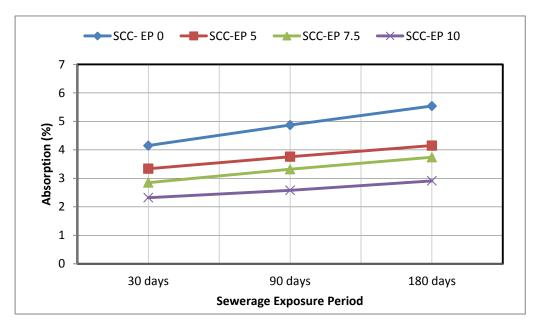
Fig. 5 : Absorption of epoxy modified SCC mixes exposed to sewerage
