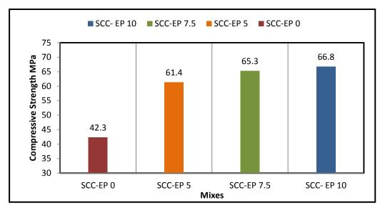
Fig. 1 Compressive strength of various types of SCC-EP at 28 days water curing
