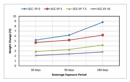
Fig. 4 : Weight change of epoxy modified SCC mixes exposed to sewerage
