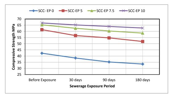
Fig. 2 Compressive strength of epoxy modified SCC mixes exposed to sewerage
