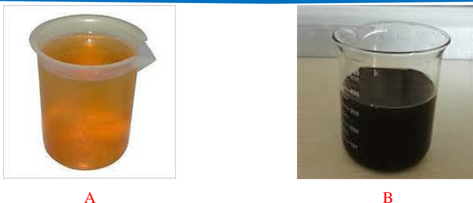
Fig. (4): Sulfonated LAB produced from: (A) good LAB and (B) from bad LAB
