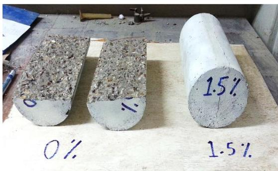
a) Comparison between the specimen of the highest (PET) fibers percentage and the reference after the test directly.
