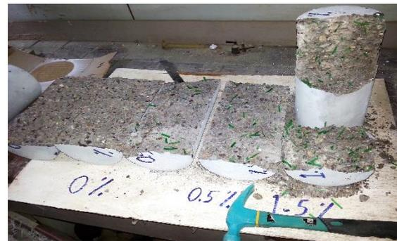
b) After hitting the specimen by the hammer for more than (136) times, it was separated a small part from the cylinder that contains the fibers percentage (1.5%).
