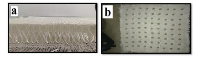
Plates (1): 3D textile glass fiber made in china; a) Zoom view. b) Holes made in 3D glass fiber.
