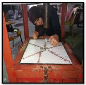
b) Crack width measuring by Vernier Caliper
