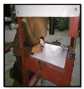
a) Crack width measuring by Portable Microscope.
