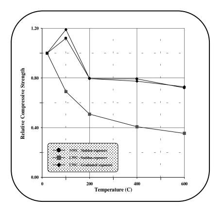
Fig. (5 )Relative Compressive strength-temperature relationships of SLWC and NWC at 28 day
