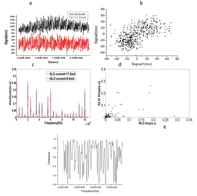
**Figure(2)** Synchronization of bidirectionally coupled two chaotic oscillators ,a:time series ,b:correlation diagram(in phase),c:FFT of MLD(blue trace) and SLD(red trace) signals ,d: FFT, and e:the coherence. amplitudes correlation of MLD and SLD signals in case of  $I_{MLD}$  =8.9mA and  $I_{SLD}$ =17.5mA
