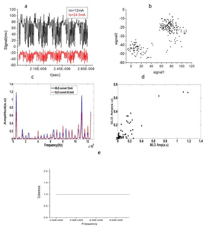
**Figure**(4)Synchronization of bidirectionally coupled two chaotic oscillators in case of I<sub>MLD</sub>=12mA and I<sub>SLD</sub>=24.3mA.( a:time series ,b:correlation diagram(in phase),c:FFT of MLD(blue trace) and SLD(red trace) signals ,d: FFT, and e:the coherence).
