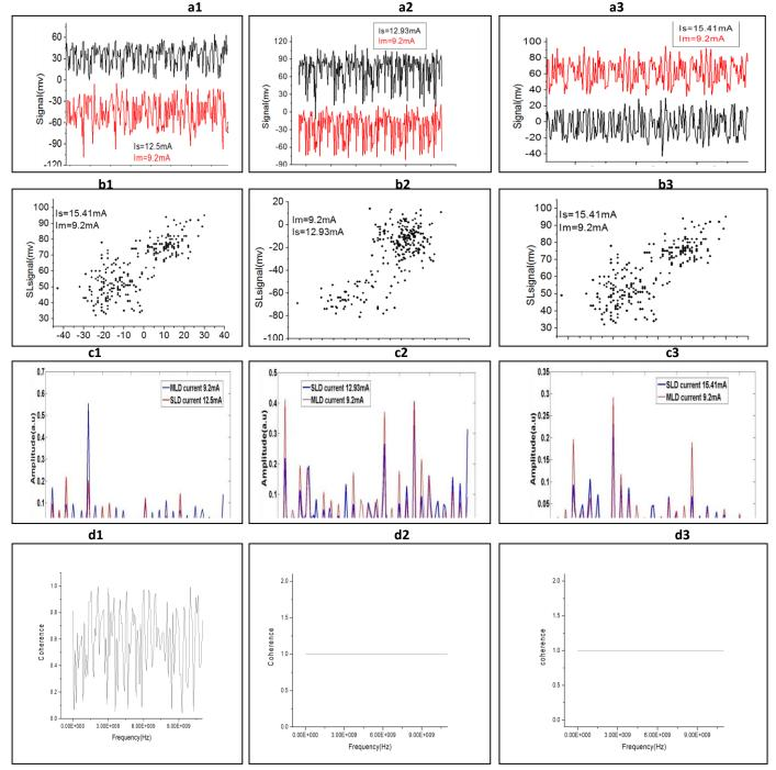
Figure(5):(a1-a3) oscilloscope traces of MLD and SLD signals red and black respectively. (b1-b3)Phase form(correlation diagram),( c1-c3) FFT( d1-d3) coherence of MLD and SLD signals red and blue respectively in all cases, and I<sub>MLD</sub>=9.2mAwhile for a1: I<sub>SLD</sub>=12.5mA, a2: I<sub>SLD</sub>=12.93mA and for a3 : I<sub>SLD</sub>=15.41mA.
