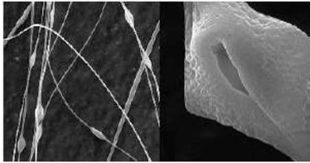
**Figure 3: SEM images of surface coated by PA nanofibers under (34 kV)**
