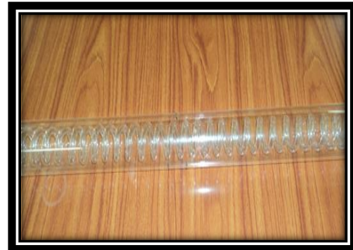
Fig .5. Test section Pyrex spiral annulus.
