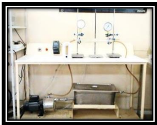
Fig .3. The Experimental system of the convective heat transfers and flow characteristics for nanofluid.
