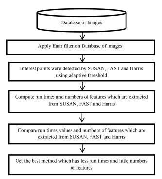
Figure 3: Block diagram of proposed system for feature extraction
