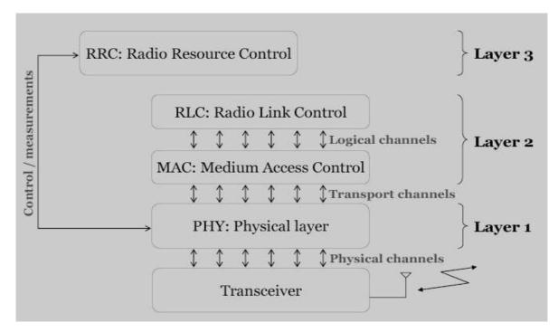
Figure 3 - LTE protocol Architecture.
