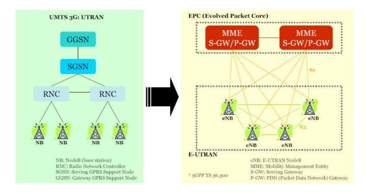
*Figure 4 – LTE Network Architecture*
