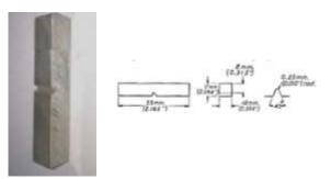
Figure 2: Charpy Impact Test Specimen (all dimensions in mm)
