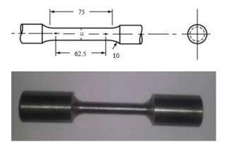
Figure 1: Tensile test specimen (all dimensions in mm)
