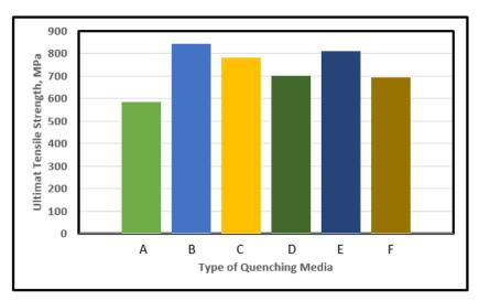
Figure 4: The effect of varying quenching media on ultimate tensile strength
