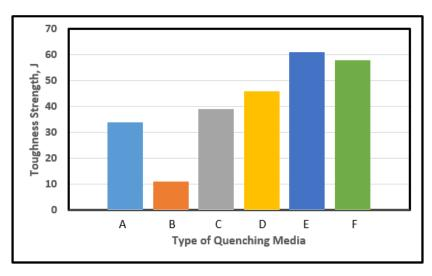
Figure 5: The effect of varying quenching media on toughness
