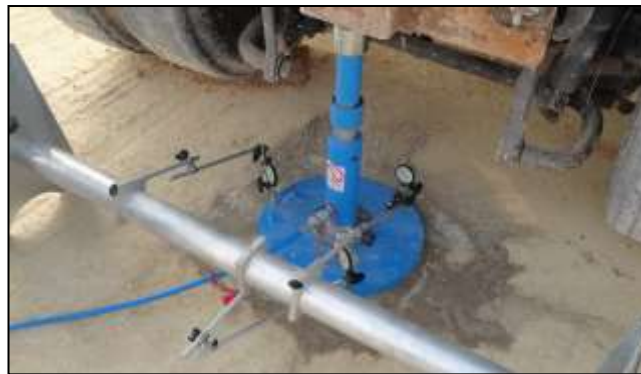
Fig. 2. Static Plate Load Test (PLT).
