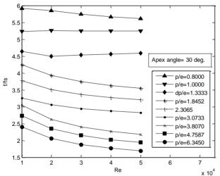
Fig. 10: Friction factor ratio vs. Reynolds number at various p/e ratio and at apex angle α=30 deg.
