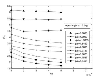
Fig. 9: Friction factor ratio vs. Reynolds number at various p/e ratio and at apex angle  $\alpha$ =10 deg.
