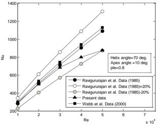
Fig. 12: comparison of present numerical results with previous workers at helix angle  $\beta$ =70 deg., apex angle  $\alpha$ =10 deg., fin height e=0.8 mm
