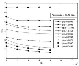
Fig. 11: Friction factor ratio vs. Reynolds number at various p/e ratio and at apex angle α=53.13 deg.
