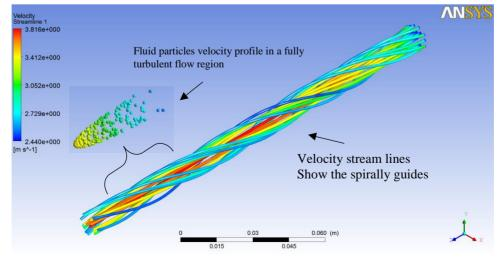
Fig. 7: Fluid particles velocity shape in a fully turbulent flow region and the velocity streamlines for the flow at Re=30000,  $\beta$ =70 deg.,  $\alpha$ =0 deg.,  $\alpha$ =0 mm.
