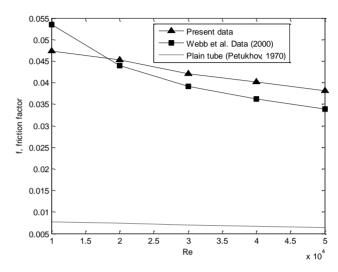
Fig. 13: comparison of present numerical results with previous workers at helix angle  $\beta$ =70 deg., apex angle  $\alpha$ =10 deg., fin height e=0.8 mm.
