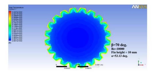
Figure 2: flow temperature distributions along internally finned tubes with various parameters.
