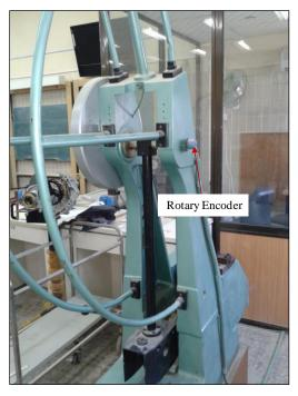
Fig. 2 Impact Testing Apparatus
