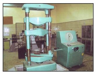
Fig. 1 Universal Testing Machine ZD100.
