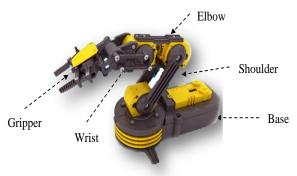
Fig.11 Body of the robot manipulator
