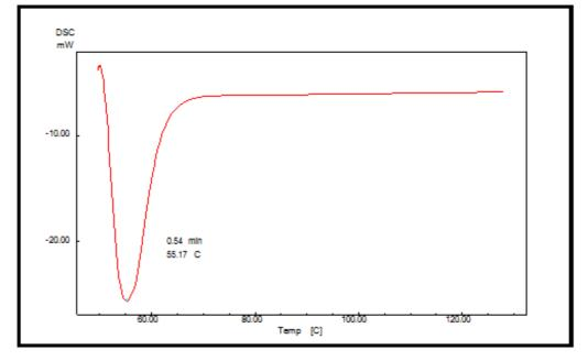
Figure 5. DSC thermogram of pure Poloxamer
