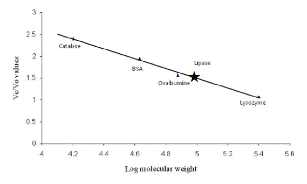
Figure 6: Determination of the molecular weight of lipase.
