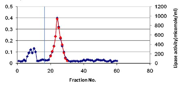
Figure 2. Lipase Ion exchange chromatography through DEAE-Cellulose column  $(3\times8)$  cm. The column was calibrated with phosphate buffer saline PBS 0.1 M and pH 7.0, flow rate 40 ml/hour and 5ml / fraction.
