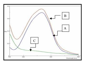
Fig. 2: Absorption spectra of 100 μg salbutamol sulphate/10 ml treated according to the recommended procedure and measured against (A) blank, (B) distilled water and (C) blank measured against distilled water.
