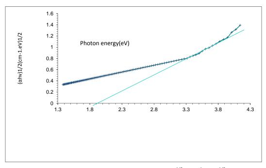
Figure (4) the relationship between (αhv)<sup>1/2</sup>(cm<sup>-1</sup>.eV)<sup>1/2</sup> and photon energy of PVA-Ni composites for 50wt.% Ni
