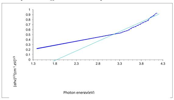
Figure (7) the relationship between (αhv)<sup>1/3</sup>(cm<sup>-1</sup>.eV)<sup>1/3</sup> and photon energy of of PVA-Ni composites for 50wt.% Ni
