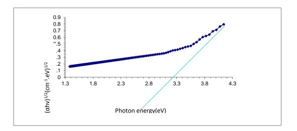
Figure (2) the relationship between  $(\alpha hv)^{1/2}$  (cm<sup>-1</sup>.eV)<sup>1/2</sup> and photon energy of pure polymer (PVA).
