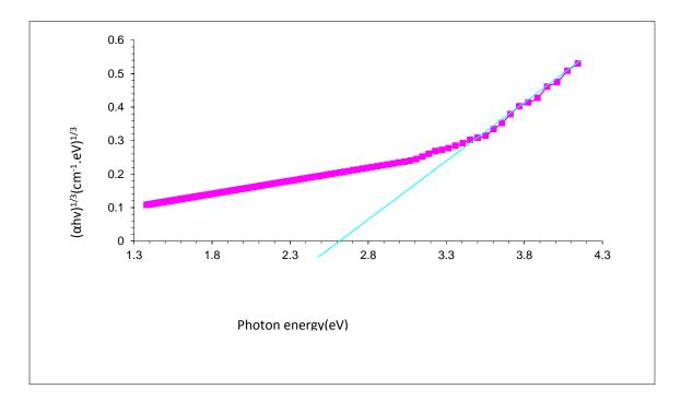
Figure (5) the relationship between  $(\alpha hv)^{1/3}(cm^{-1}.eV)^{1/3}$ and photon energy of pure polymer (PVA).
