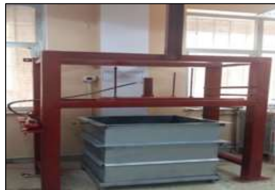
Plate 2: The steel frame with hydraulic compression handle jack
