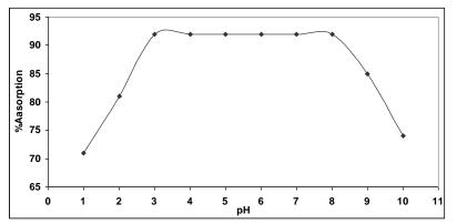
Fig. 3 The effect of pH on the percentage of adsorption
