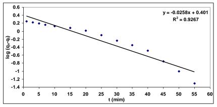
Fig. 10 Pseudo-first-order kinetic for adsorption Ni(II) on GTW
