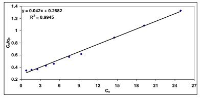
Fig. 7 Linear form of Langmuir equation for adsorption Ni(II) on GTW
