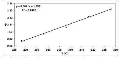
Fig. 4 The effect of temperature on the adsorption capacity
