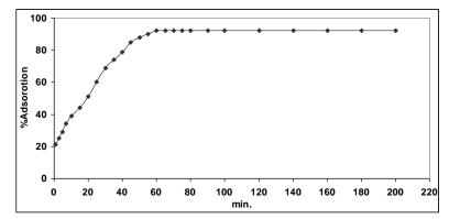
Fig. 2 The effect of contact time on the percentage of adsorption
