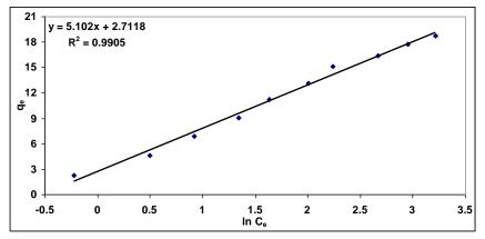
Fig. 9 Linear form of Tempkin equation for adsorption Ni(II) on GTW
