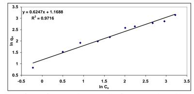
Fig. 8 Linear form of Freundlich equation for adsorption Ni(II) on GTW
