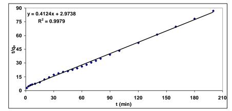
Fig. 11 Pseudo-second-order kinetic for adsorption Ni(II) on GTW
