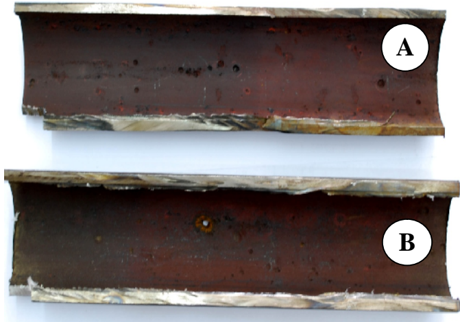
Figure (2): A-Longitudinal cross section of damaged and undamaged boiler pipes. B- Half rings samples taken from each pipe.
