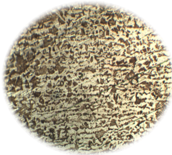
Figure (6): Micrograph structure of the un-failed pipe no. 6/93, (200X)
