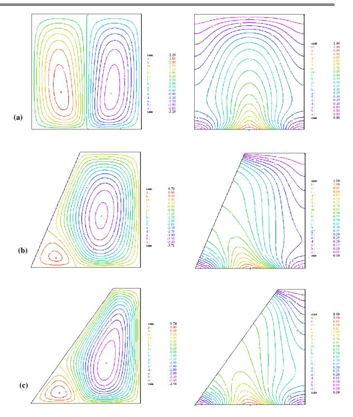
Fig.4 Streamlines (left) isotherms (right) at Ra=100 a) AR=1 b) AR=0.45 c) AR=0.25
