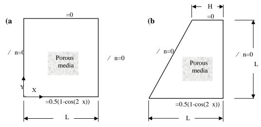
Fig.1 Schematic diagram of the physical domain a) square cavity b) trapezoidal cavity
