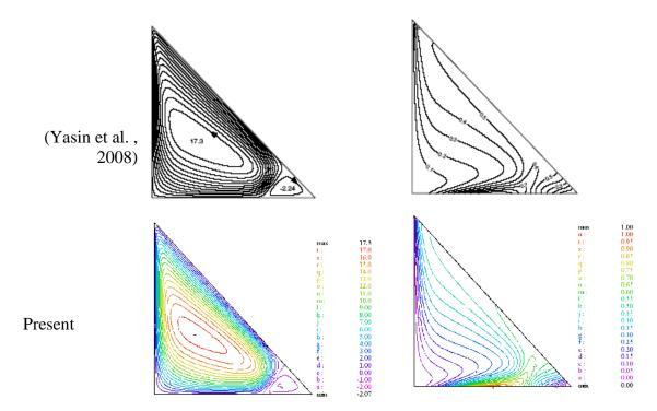
Fig. 3. Comparison of streamlines and isotherms at Ra =1000 with results of (Yasin et al.,
