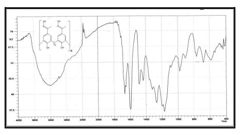
Figure (3.4) The FTIR spectra of (PHAO1)
