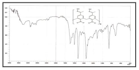
Figure (3.6) The FTIR spectra of (PNAO1)
