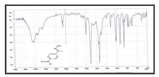
Figure (3.2) The FTIR spectra of (Oxime 2)
