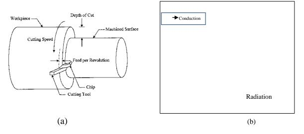
**Fig.(1)** Turning process (a) Basic cutting parameters (**Yang**, **1998**). (b)Thermal fields (Abukhshim, 2006).
