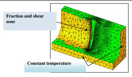
Fig. (2) Boundary conditions on the workpiece.
