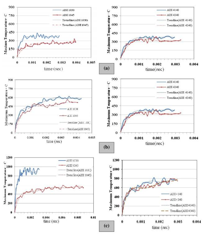
**Fig. (5)** Comparison of temperature response in early and beginning of steady stages for workpieces used;
