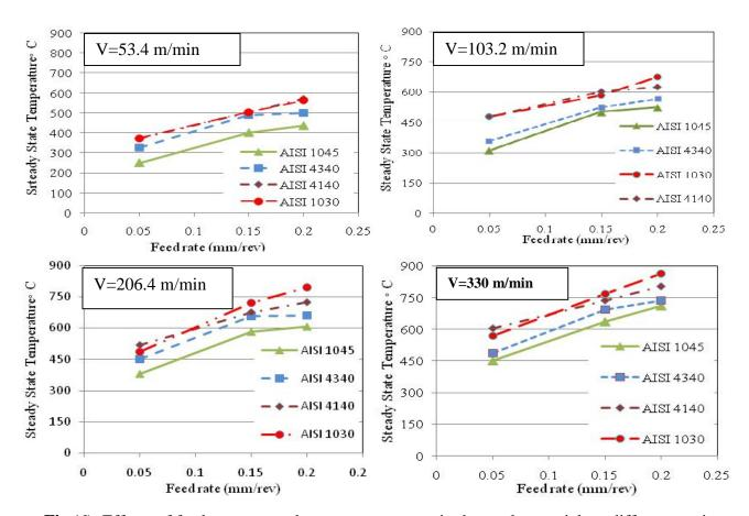
**Fig.(6)** Effects of feed rate on steady-state temperature in the work materials at different cutting speed
