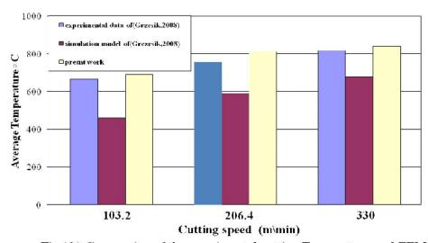
Fig.(3) Comparsion of the experimental cutting Temperature and FEM simulated values of (Grzesik,2008) with FEM simulation model in presnt work
