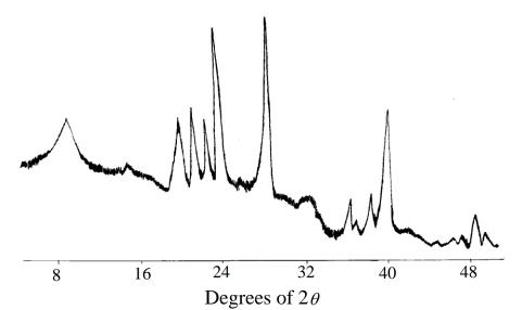
Fig. (1): Powder x-ray Diffraction Pattern of Natural Clay Sample .
