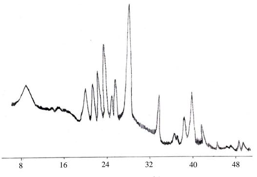
$\label{eq:Degrees} Degrees \ of \ 2\theta$  Fig. (2): Powder x-ray Diffraction Pattern of Grafted Clay Sample .
