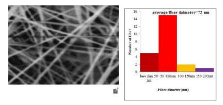
Figure (3): (a) SEM image of 0.8 wt. % MWCNT/ Nylon 6 nanofibers membrane, (b) fiber diameter distribution.
