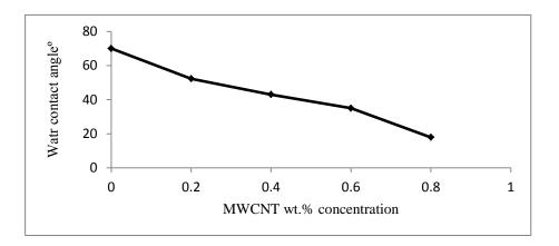
Figure (4): Water contact angle variations of various (Nylon / MWCNT) electrospun nanofibrous membranes.
