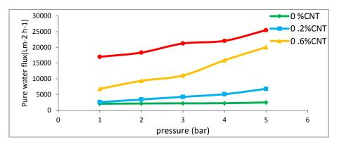
Figure (6): Effect of membrane pressure on the pure water permeation flux of the Nylon 6/MWCNT nanofiber membrane at room temperature and 50 min time.
