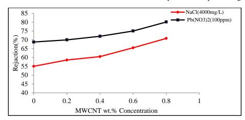
Figure (7): Effect of MWCNT/Nylon 6 ratio on rejection of Pb  $(NO_3)_2$  salt and NaCl salt aqueous solutions with initial concentration 100 ppm and 4000mg/L respectively, at room temperature and 1 bar.
