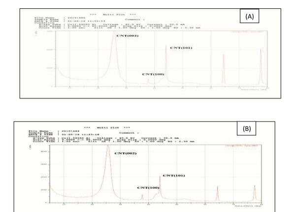
Figure (1): X-ray of (A) raw carbon nanotube, (B) acidic modification carbon nanotube by ((1/3)  $HNO_3/H_2SO_4$ ).
