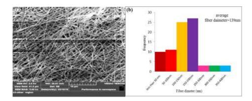
Figure (2): (a) SEM image of pure (Nylon 6) nanofibers membrane, (b) fiber diameter distribution.
