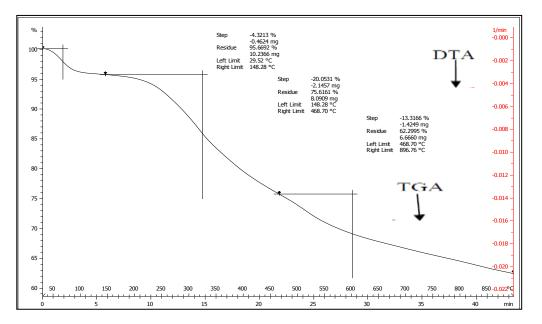
Fig. 2: Thermogravimetric analysis (TGA)/differential thermal analysis (DTA) for RHAC-Pd(DTO)<sub>2</sub>.Three characteristic decomposition stages are shown.
