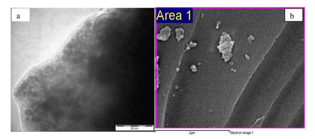
Fig. 5: (a) The TEM image of RHAC-Pd(DTO)<sub>2</sub> at ca. 50 nm, showing the irregular pore arrangements. (b) The SEM image, showing a small degree of pore arrangement.
