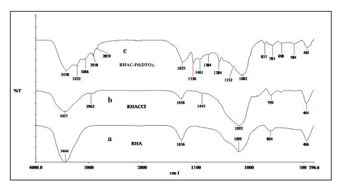
Fig.4: The FT-IR spectra of **a** RHA, **b** RHACCl and **c** RHAC-Pd(DTO)<sub>2</sub>
