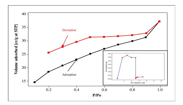
Fig.1: The nitrogen adsorption–desorption isotherms of RHAC-Pd-(DTO)<sub>2</sub>. The inset shows the corresponding pore size distribution.
