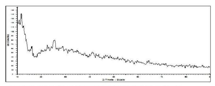
Fig. 3: The X-ray diffraction pattern shows amorphous nature of RHAC-Pd(DTO)2
