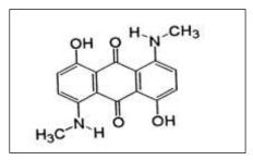
Figure 1: The structure formula of dispersive blue 26 dye.
