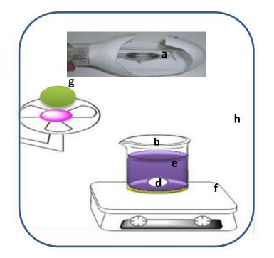
Scheme1. Schematic diagram of photo-reactor components. Whereas, a) (250 W) High pressure mercury lamp,(b) 400 cm<sup>3</sup> Pyrex glass beaker, (c) dispersive blue 26 dye with ZnO as suspension solution, (d)Teflon bar, (e)suspension solution (Dye with photo-catalyst), (f) magnetic stirrer, (g) fan and (h) wooden box.
