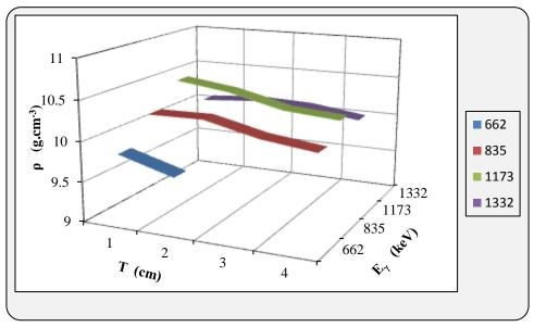
Fig.9: density distribution vs. thickness of alloy at particular energy.
