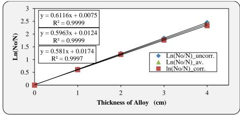
Fig.5: shows linear attenuation data versus thickness of MCP-96 alloy for 1173 keV of gamma rays energy.
