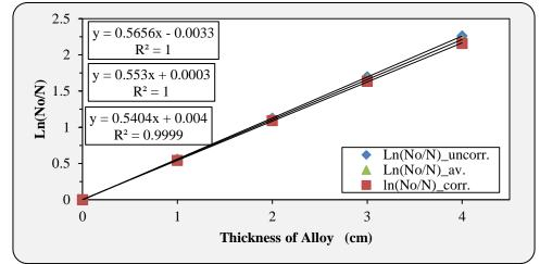
Fig.6: shows linear attenuation data versus thickness of MCP-96 alloy for 1332 keV of gamma rays energy.
