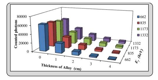
Fig.2: the dependency of counted photons on the thickness of alloy vs. the energy of incident gamma rays.
