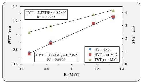
Fig.8: half and tenth -value thickness (HVT) and (TVT) for MCP-96 alloy vs. gamma ray energy.
