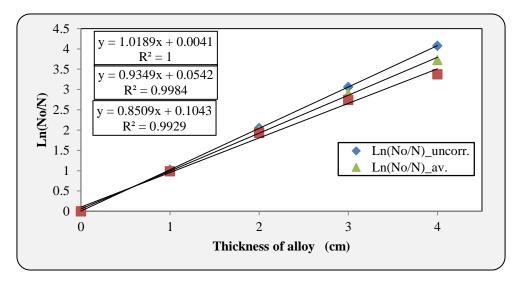
Fig.3: shows linear attenuation data vs. thickness of MCP-96 alloy for 662 keV of gamma rays energy.
