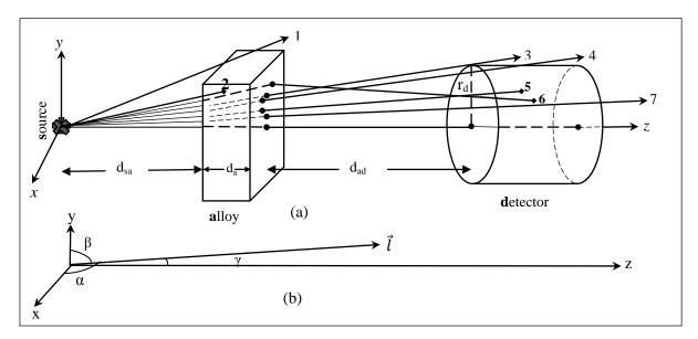
Fig.1: Geometrical configuration simulation of source-alloy, alloy-detector systems by present Monte Carlo computer program. (a) Fixed dimensions system and (b) reference dimensions system.
