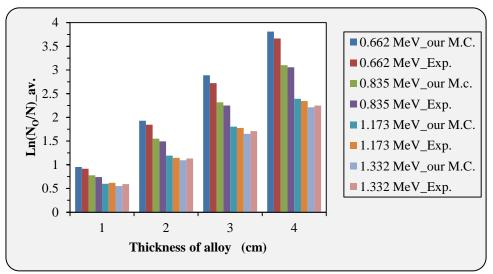
Fig.7: our Monte Carlo results of attenuation data compared to published experimental results for varies energies of gamma rays.
