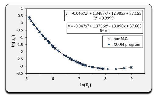
Fig.10: log-log axises of gamma energy vs. simulated (\*) and calculated (•) values of mass attenuation coefficient for MCP-96 alloy.
