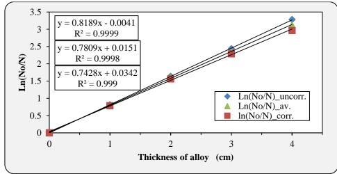
Fig.4: shows linear attenuation data versus thickness of MCP-96 alloy for 835 keV of gamma rays energy.
