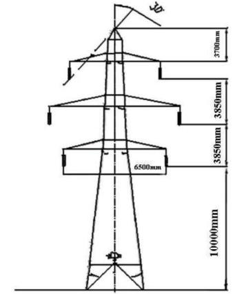
Figure (1) Double circuit 132 KV power line (MOE, 2006 and Alkhazraji, 2011)
