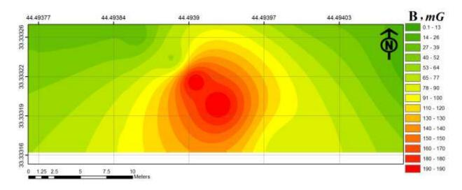
Figure (3) Magnetic field distribution in Al-Mashtal substation power network
