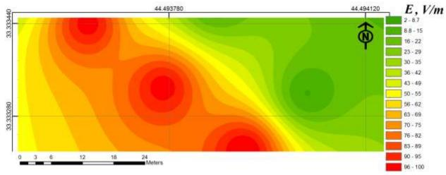
Figure (2) Electric field distribution in Al-Mashtal substation power network
